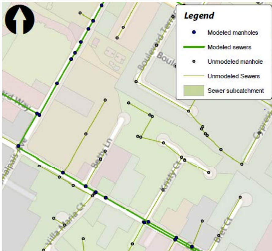
Figure 3-3: Example Sewer Subcatchments
